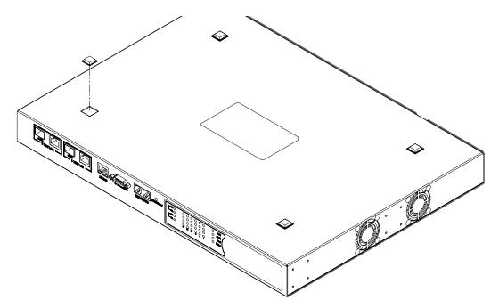
Figure 4-3. Attaching the Adhesive Feet
